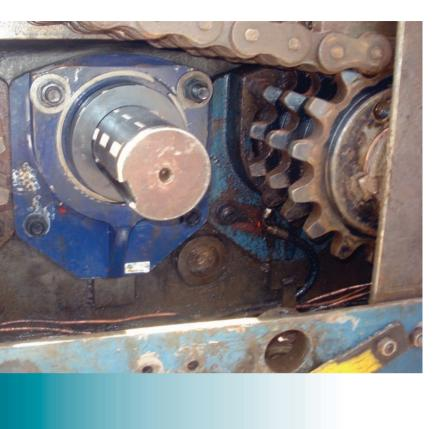
Still operating seven months later, the Timken flange block continues to work like new. The triple-lip seal keeps contaminants out and is proving to be superior to the competing bearing. The unit handles more than two times the weight of the old bearing, with an expected design life of 100,000 hours.
